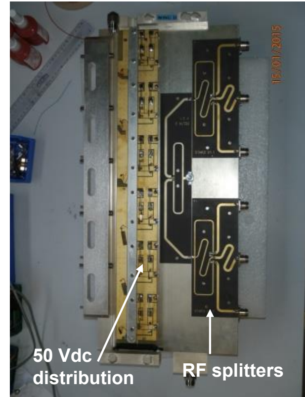
Water cooled wing with 6 RF modules, developed at ESRF
