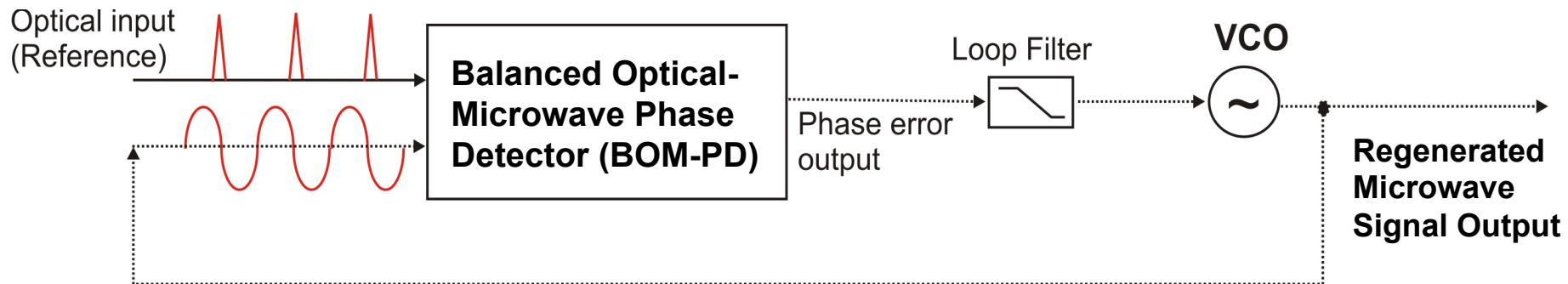
Tight locking of modelocked laser to microwave reference
