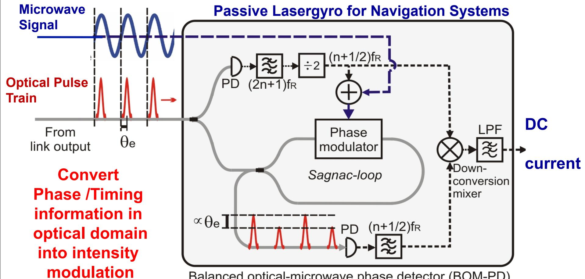
Electro-optic sampling of microwave signal with optical pulse train
