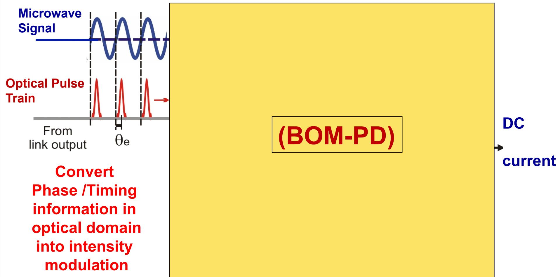
Electro-optic sampling of microwave signal with optical pulse train
