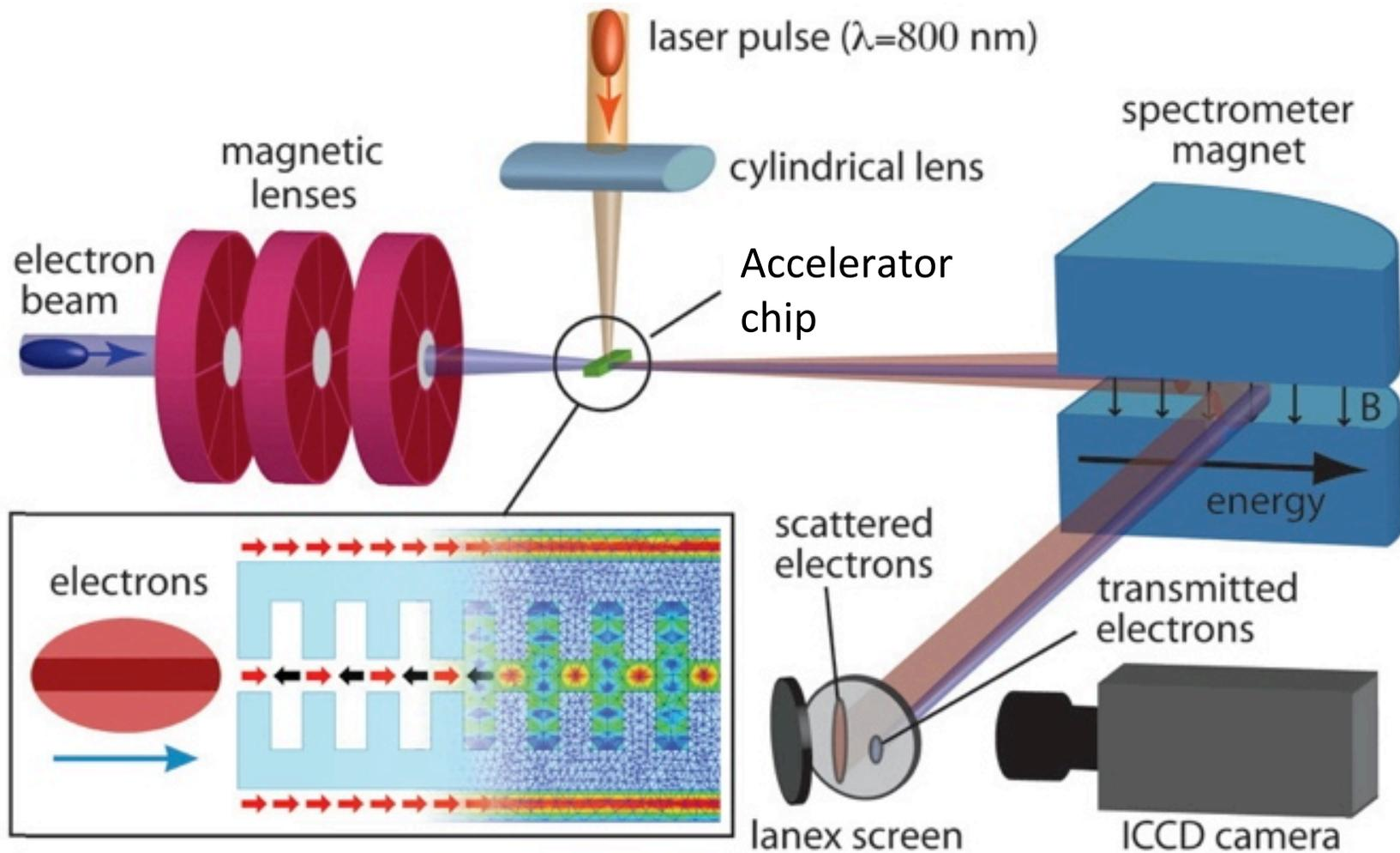
Gradients in the first experiment were 10 times higher than the main SLAC linac.
