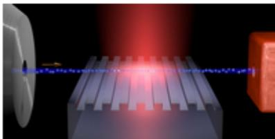
In a new technique, light pulses accelerate electrons in a compact particle accelerator.
