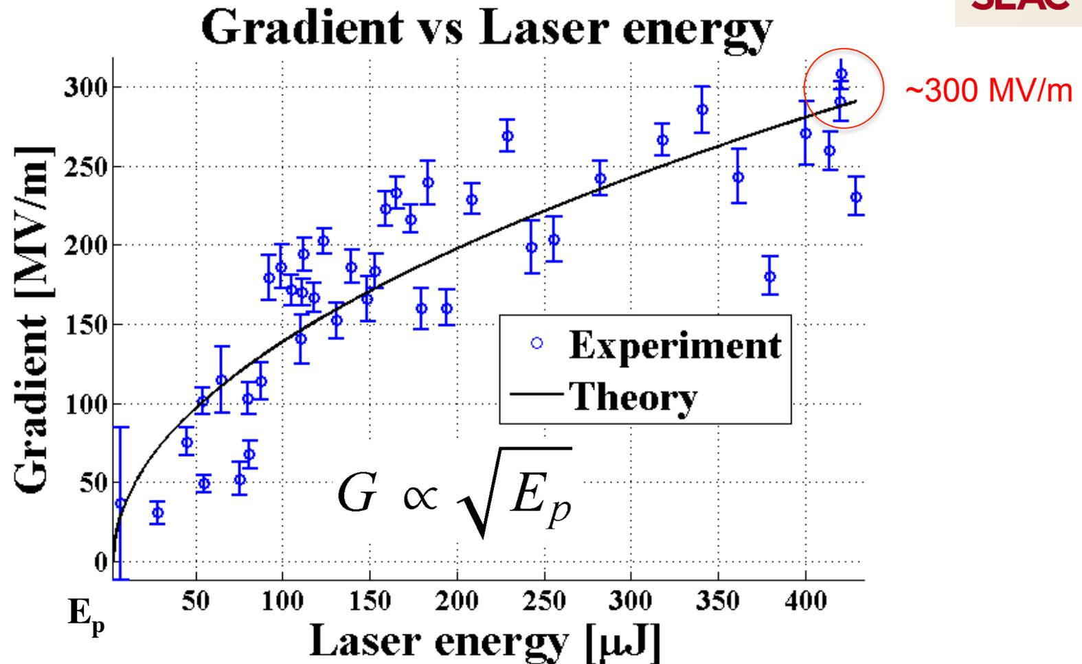
With further optimization of the structure designs, GV/m level gradients should be achievable
