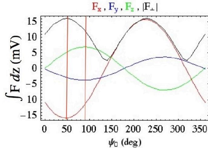
Harmonic analysis of one undulator period driven by two lasers:
