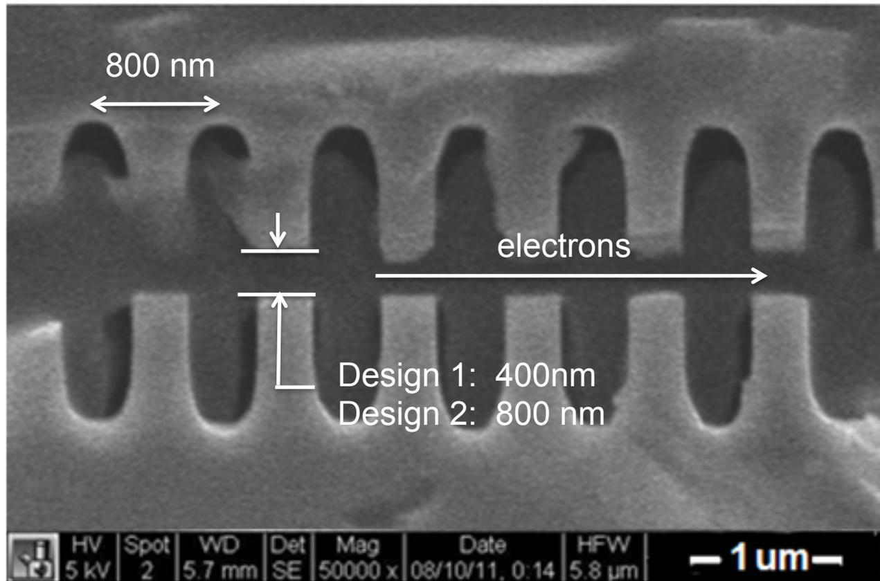
Electron microscope image of the bonded structure.
