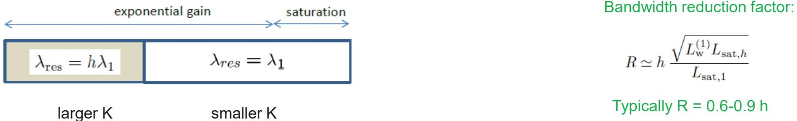
The fundamental and all harmonics have to stay well below saturation in the first part of the undulator. Use of phase shifters in the first undulator is optional.
