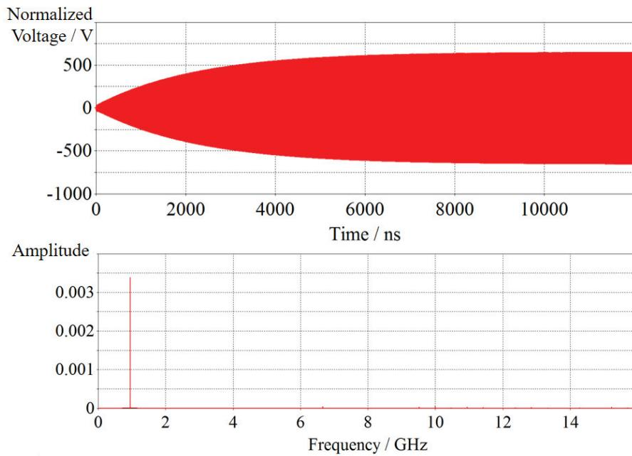
The output signals in time domain and in frequency domain of the second harmonic cavity (0.952GHz).
