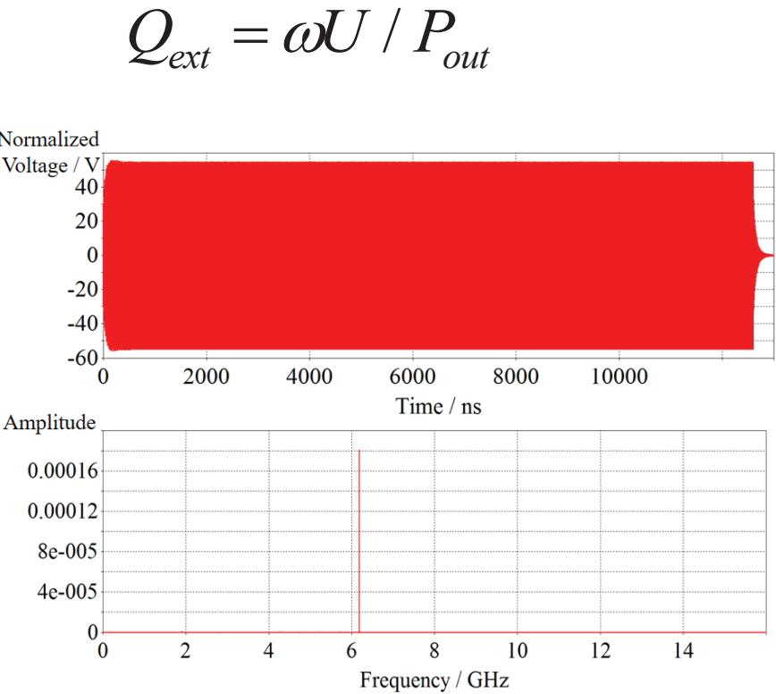
The output signals in time domain and in frequency domain of the thirtieth harmonic cavity (6.188GHz).
