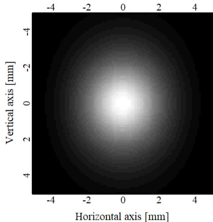
1% rms energy spread; Divergence and Beam size (1 mrad, 1mm)
