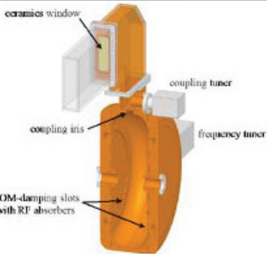
Figure 1: Structure of the new HOM-damped cavity.
