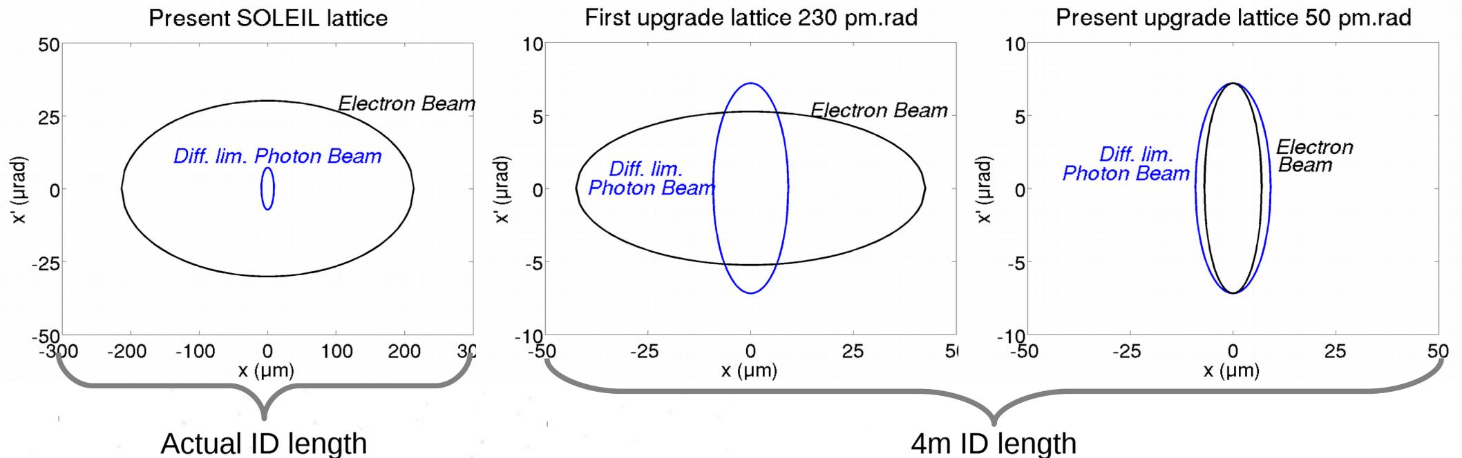
Diffraction limited photon beam emittance is 65 pm.rad at an energy of 3 keV
