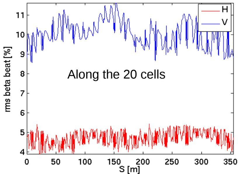
Simple error quad strength by 1‰ rms, 500 trials
