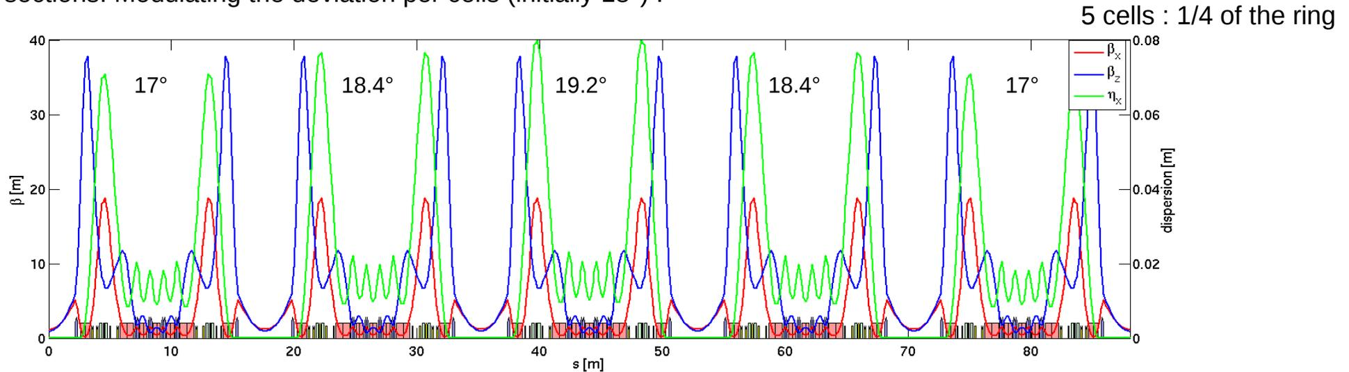
Keeping sextupole and octupole strengths, the beam dynamics is ~unchanged. Emittance increase is marginal
