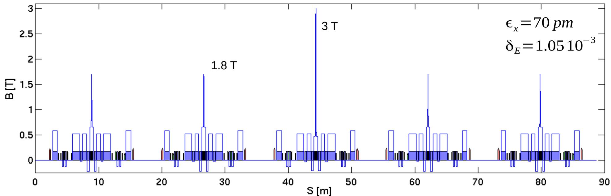
Add 1.8 T on central bend of other cells to reduce back the emittance  $\sim 70 \text{ pm.rad}$
