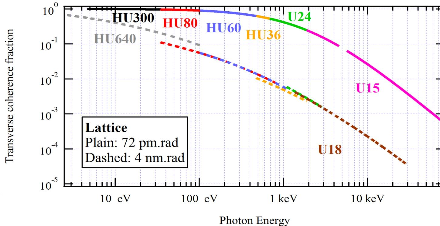
The photon beam should be fully coherent up to almost 200 eV, exceeding 40 % at 1 KeV
