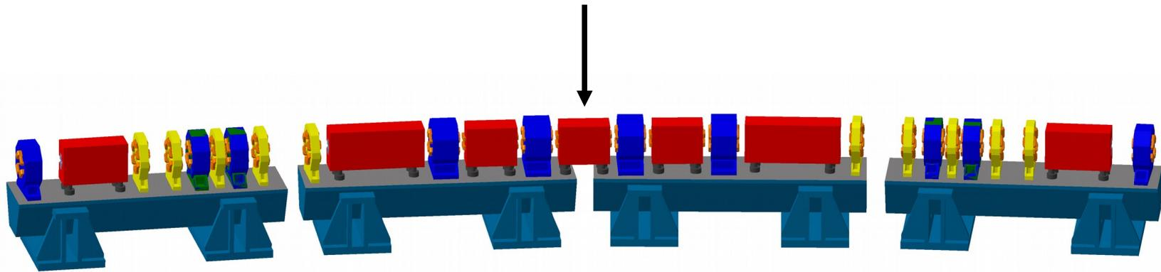
Insertion of 3T super-bend in the central magnet of the cell
