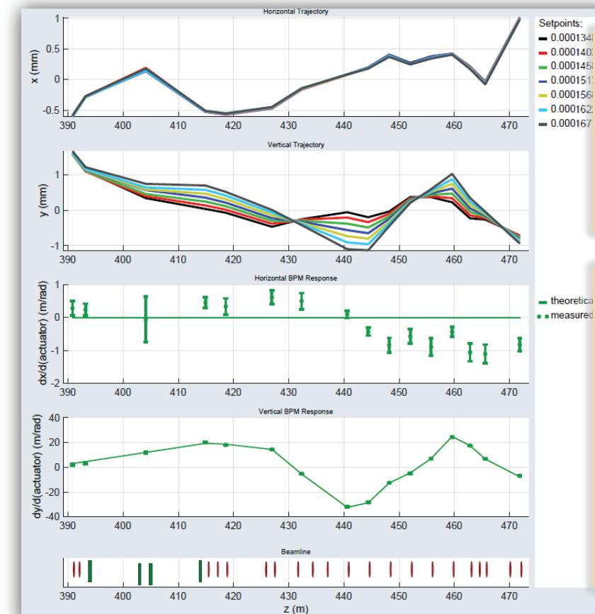
Horizontal and vertical orbits of all measurement steps
