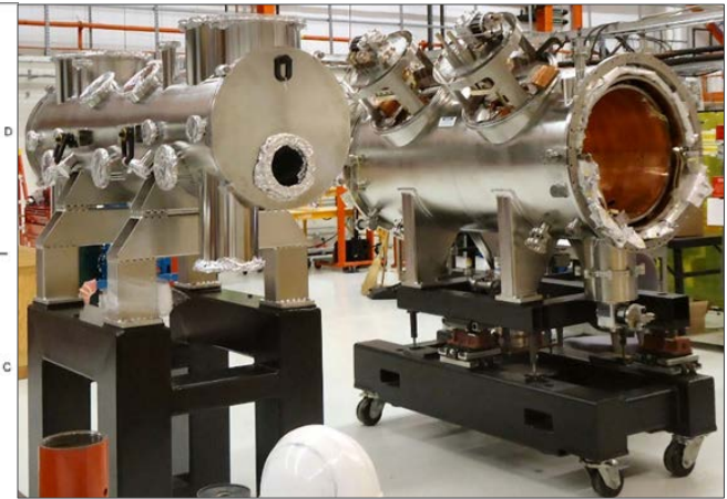
HSCU cryostat developed by APS
