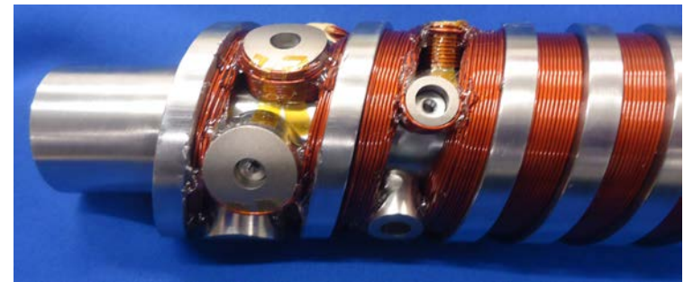
HSCU prototype coil winding showing end detail.
