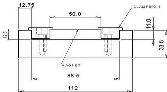
Figure 11: 1m PPM undulator design from side view.
