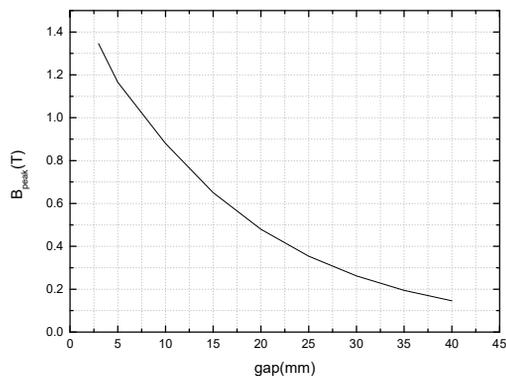
Figure 14: Peak magnetic field at different gaps.
