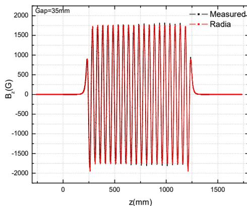
Figure 16: Magnetic field profile for the gap of 35mm.
