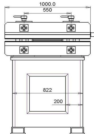
Figure 12: 1m PPM undulator with support structure.
