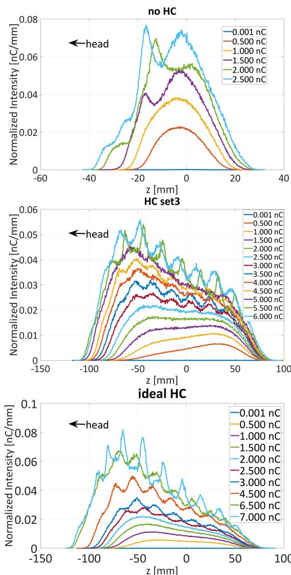
Figure 5: Bunch final distributions under different settings of the harmonic cavities at different single-bunch charges.
