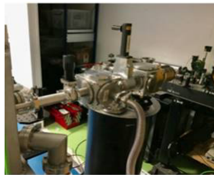
Figure 11: CCD camera installed 3 m from the exit of the undulator.
