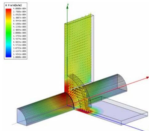
"Position" cavity (dipole TM11 mode but no monopole
