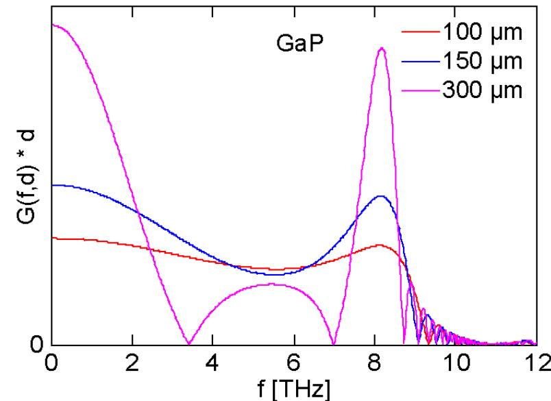
$$G(f, d) = \frac{2}{1 + n(f) + i\kappa(f)} \frac{1}{d} \int_0^d \exp \left[ i 2\pi f z \left( \frac{1}{v_{ph}(f)} - \frac{1}{v_g} \right) \right] dz$$
