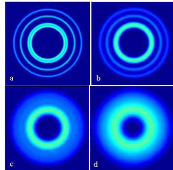
Simulated aluminum-foil diffraction patterns from beams with divergences of (a) 0.05, (b) 0.1, (c) 0.2, and (d) 0.3 mrad
