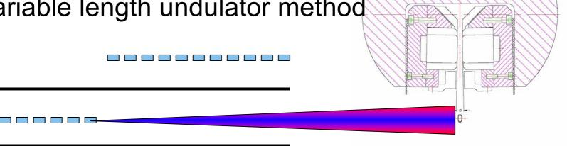
SR and FEL radiation are both "turned off" by removing segments
