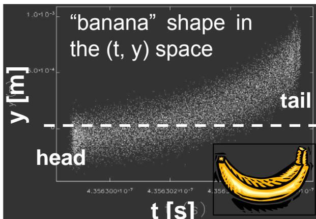
“Banana” shapes (in x and y plane) for 120 trajectories in the Linac. The bunch tail deviates from the head of about  $6 \sigma_{x,y}$  at the Linac end.
