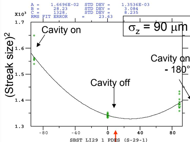
Asymmetric parabola indicates incoming tilt to beam
