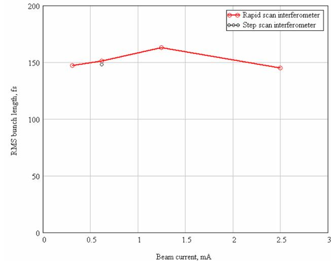
The bunch length does not change with beam current.
