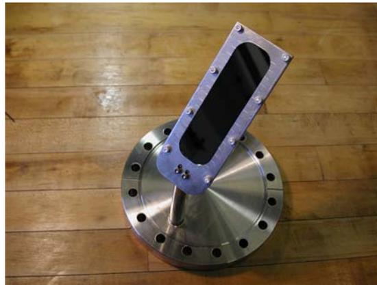
Si wafer fixed for spectrometer
