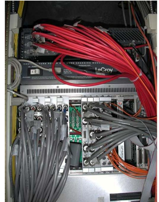
48 channels shown, 4 x 12 channel VME BLM boards shown with AMS and FSD connections on front and tube and high voltage on rear, also shown are the connections to the MPS system
