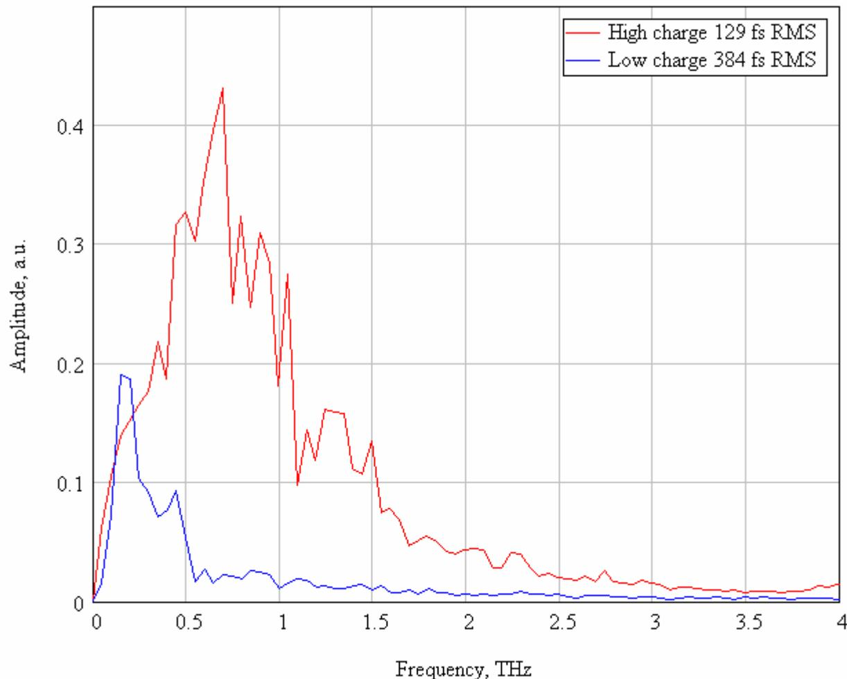
The bunch compression is optimized for the nominal (135 pC) bunch. It is also strongly bunch charge dependent.
