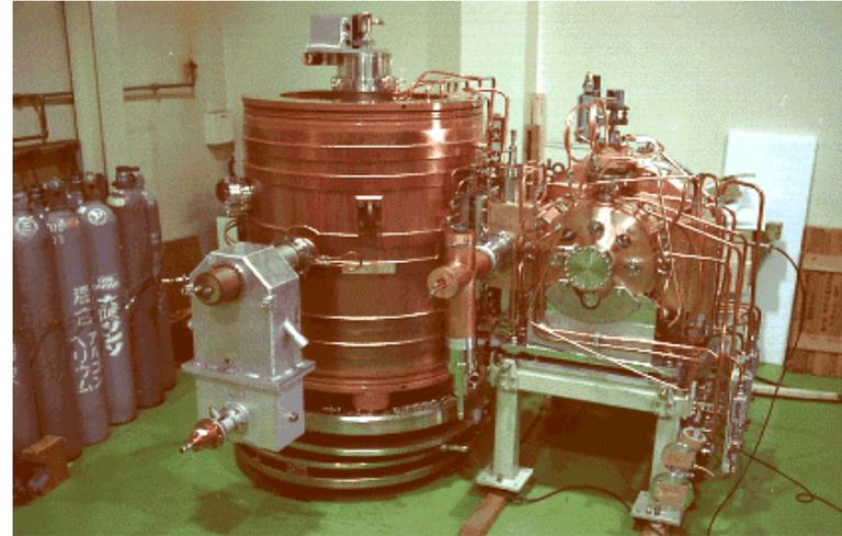
KEK ARES cavity, 509 MHz, 500 kV, 1.7 M $\Omega$
