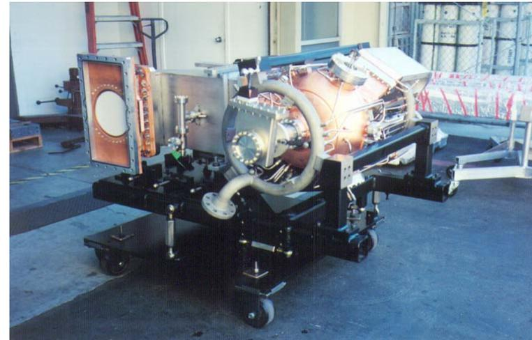
PEP-II cavity, 476 MHz, 850 kV, 3.7 M $\Omega$
