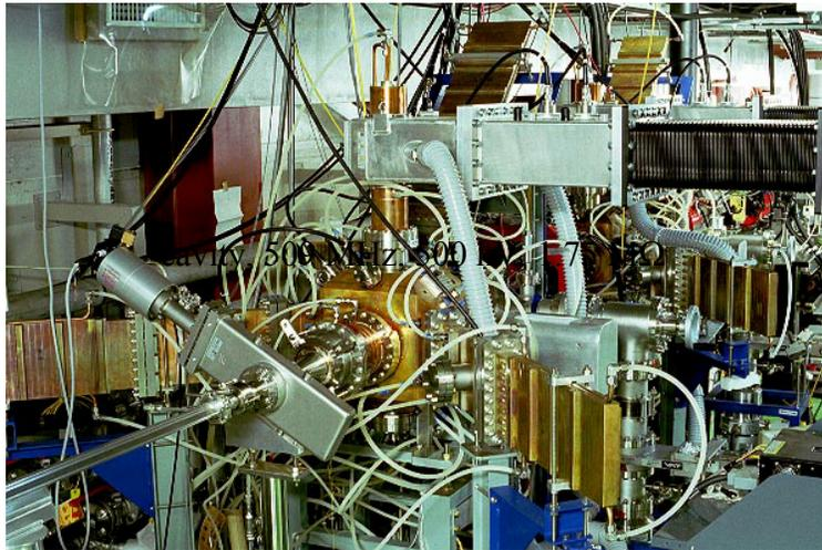
ATF cavity, 714 MHz, 250 kV, 1.8 M $\Omega$
