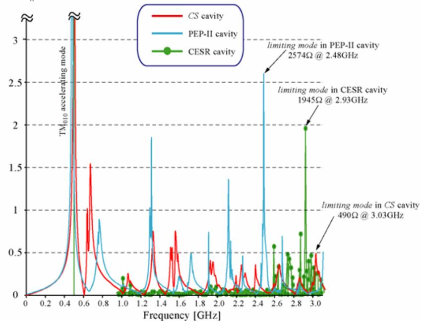
Longitudinal impedance spectra as calculated for the BESSY(CS), PEP-II and CESR cavity
