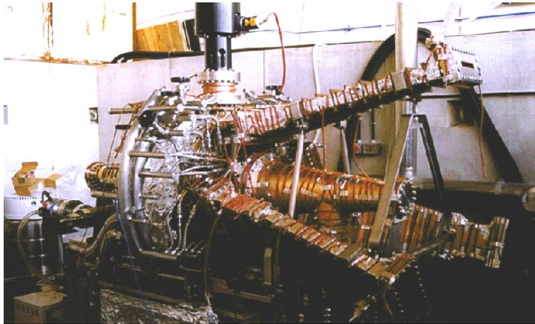
Daphne cavity, 368.26 MHz, 250 kV, 2 M $\Omega$
