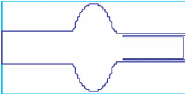
Coaxial/radial beam pipe
