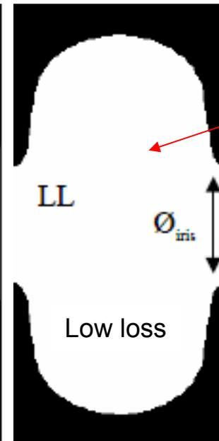
Increase the magn. volume to reduce surface magnetic field → few losses
