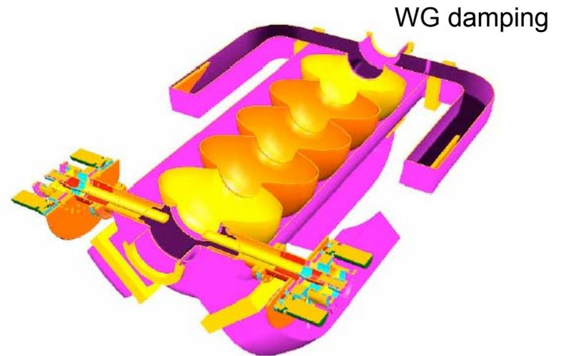
JLAB 750 MHz injector cavities: 1 A
