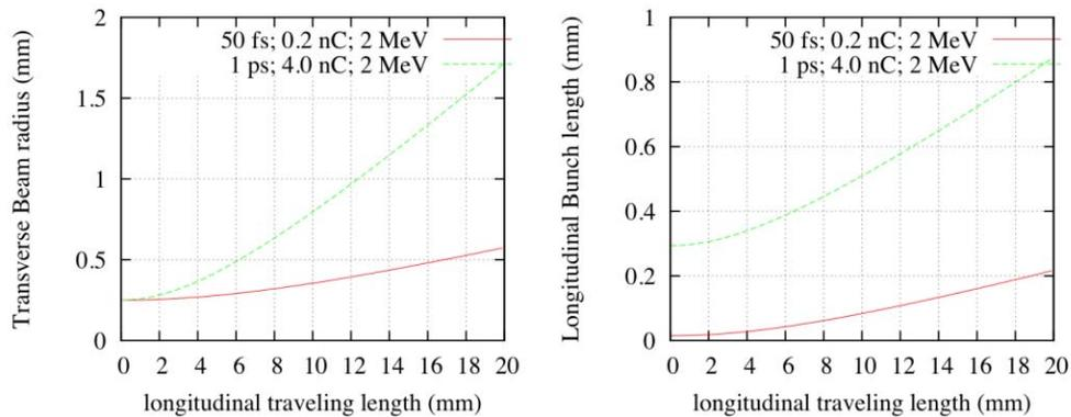
Figure1: Two beams with the energy of 2MeV and their radiuses are the same sizes of 0.25 mm. Broken line shows a beam with the time width of 1ps and the charge of 4.0nC. Solid line shows the other beam with 50fs and 0.2nC, respectively. They pass through drift space of 20mm long. Beam sizes get larger to transverse and longitudinal directions due to space charge effect.
