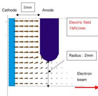
Figure 2: Electric field was calculated by the computer simulation code of MAFIA. The gap length is 2mm and the radius of the anode is 2mm. Supplied electric field is 1MV/mm. The electric field near the edge of anode plate greatly curves. Beam emittance is grown there.
