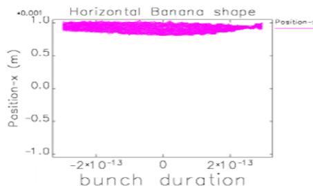
Figure 9: Jitter of the “banana” shape at the Linac end in (horizontal plane) after the trajectory bump (see, Fig.8, right). The emittance is still preserved.
