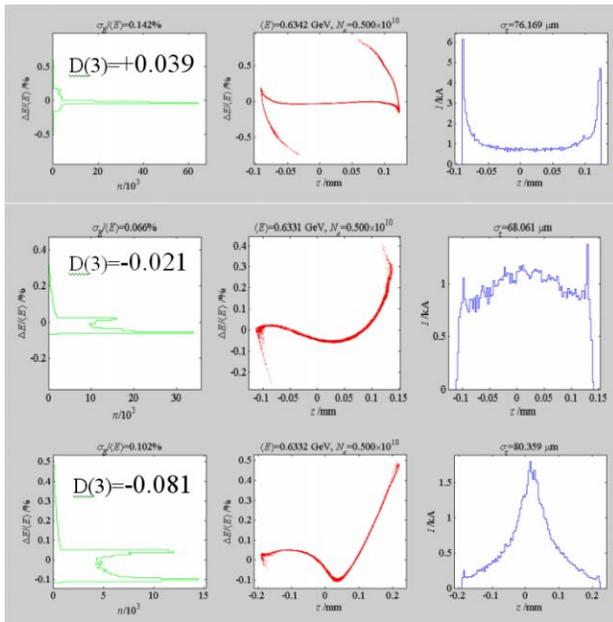
Figure 3: from left to right, energy distribution, longitudinal phase space and current profile at the Linac end. Each row of plots corresponds to a different value of the cubic energy chirp, called  $D(3)$  in units of  $0.01\text{mm}^{-3}$ . The positive sign is related to an over-compression of the bunch edges (top), while a negative sign is related to their under-compression (bottom).
