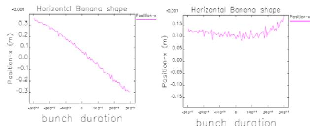
Figure 8: “banana” shape at the Linac end in the horizontal plane, before (left) and after (right) the trajectory bump. The transverse deviation of the bunch tail w.r.t. the head is reduced from 6  $\sigma_x$  to 1  $\sigma_x$ .
