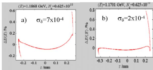
Figure 2: Longitudinal phase space at the Linac end. a) partial linearization; b) linearization improved by increasing the high harmonic cavity voltage. LiTrack [6] simulation.
