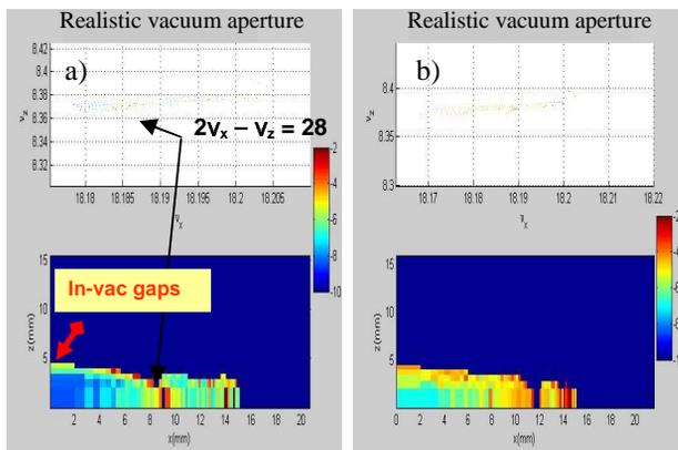
Figure 4: On-momentum dynamic aperture for a) the bare lattice and b) the lattice including an EU71 in the vertical mode where the linear tunes are not yet compensated (18.17, 8.379) and the beta beating is 12%.
