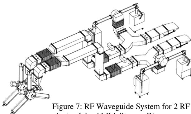
Figure 7: RF Waveguide System for 2 RF plants of the ALBA Storage Ring.
