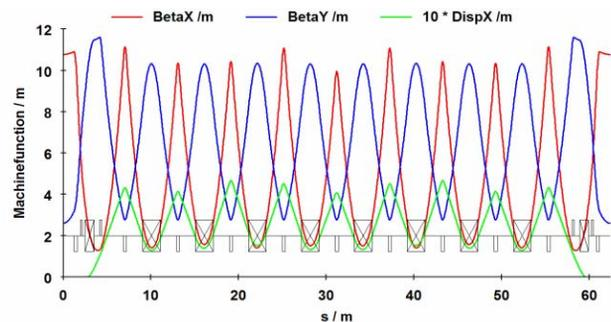
Figure 2: Lattice functions within the ALBA Booster.
