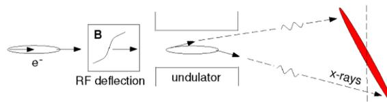
Figure 4: The chirped pulse can be slitted or compressed [11].
