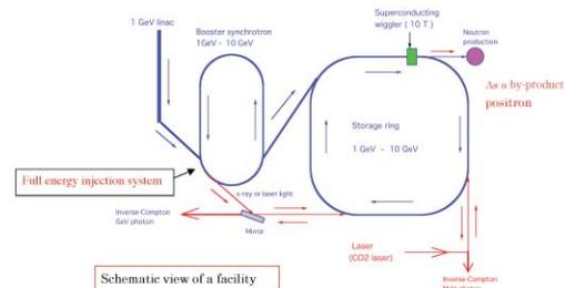
Figure 6: Schematic of multiple-wavelength facility [18].
