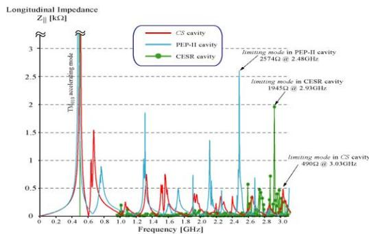
Figure 5: Comparison of  $Z_{||}$  for conventional NC cavity (PEP-II) with HOM-damped NC cavity (BESSY-CS) and SC cavity (CESR-B) [14].
