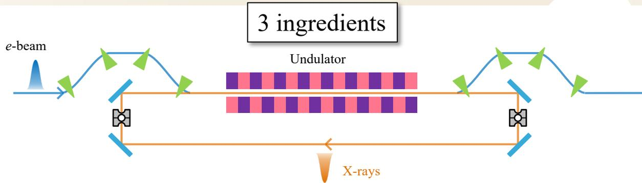
Cavity-based X-ray FELs store and recirculate the output of an amplifier in an X-ray cavity so that the X-ray pulse can interact with the following fresh electron bunches over many passes.
