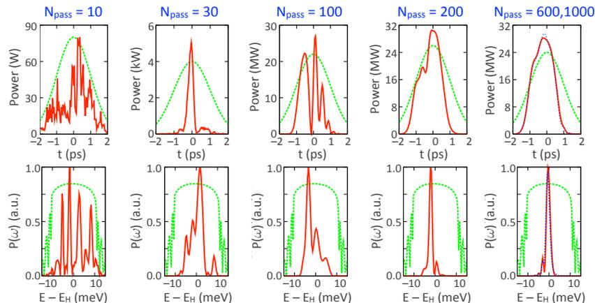
Typical longitudinal pulse evolution in an XFELO
