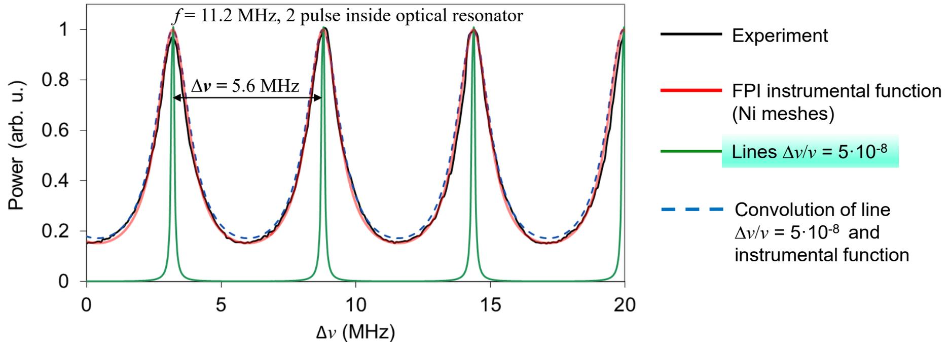
**Spectra for  $f = 5.6$  MHz (1 pulse) and  $f = 11.2$  MHz (2 pulses) are identical.
