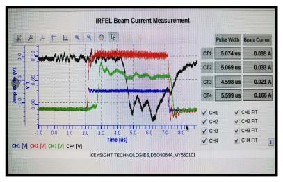
Black line: FEL signal from a pyroelectric probe
