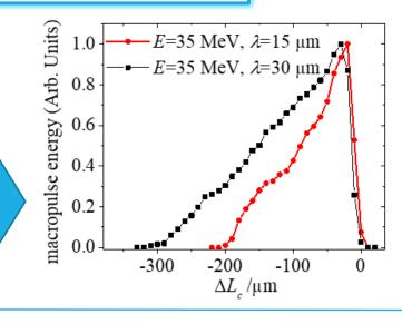
Lasing was observed over a cavity length scan range of about 10 times of radiation wavelength.
