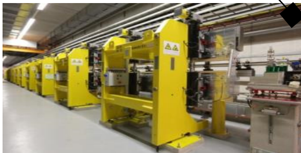
FLASH2 variable gap undulators
