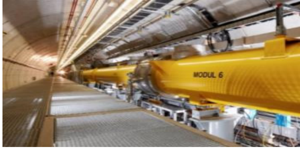
TESLA type superconducting accelerating modules 1.3 GHz
