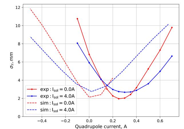
Dependence of vertical beam size at the monitor on quadrupole strength for two currents of solenoid (measurements and simulation).
