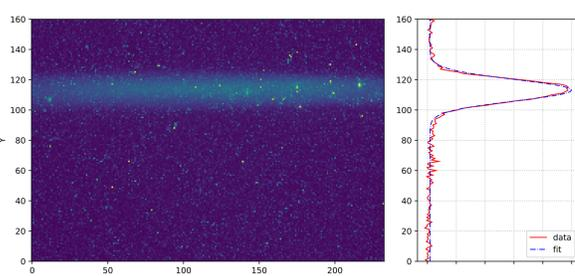
The example of beam image in a quadrupole strength variation experiment
