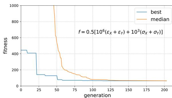
The process of optimization with DE algorithm.  $\epsilon_{x,y}$  – normalized emittance and  $\sigma_{x,y}$  – rms beam size (both in meters)
