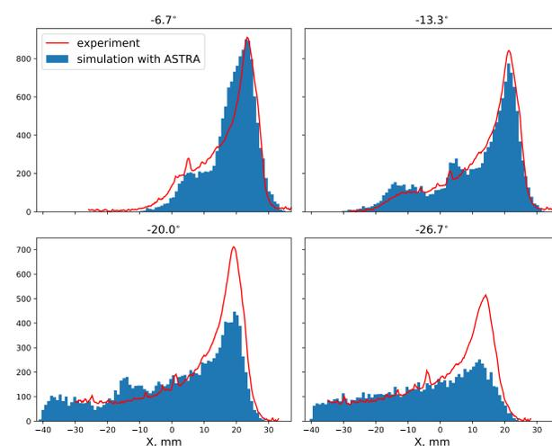
Transverse horizontal beam density distribution at the monitor for several the RF gun injection phases (0° - the phase of the maximum acceleration).
