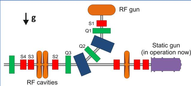
A scheme of the NovoFEL injector with the new RF gun:
