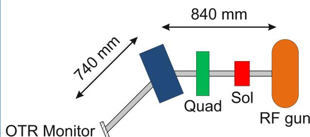
The scheme of the RF gun test stand
