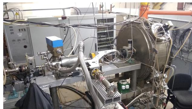
A view of RF gun stand. 90° bend is assembled.
