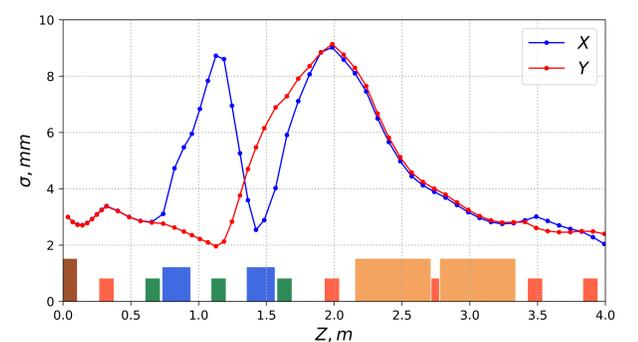
The optimized beam sizes for the RF gun beamline.
