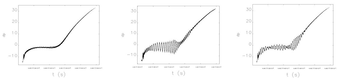
Figure 3. Longitudinal phase space of the beam at the exit of SHINE linac, with (a) 60  $\mu\text{m}$ , (b) 120  $\mu\text{m}$ , (d) 150  $\mu\text{m}$  initial density modulation
