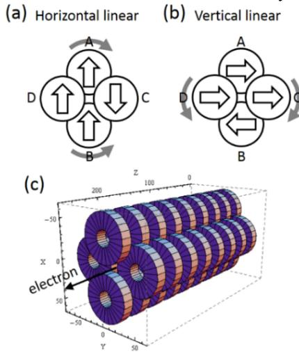
Figure 2: The configuration of four PM cylinder arrays. The rounded arrows represent the rotation direction. The operation to change the magnetic field in the (a) horizontal linear mode and (b) vertical linear mode. (c) Is a three-dimensional illustration of the PM cylinder undulator.
