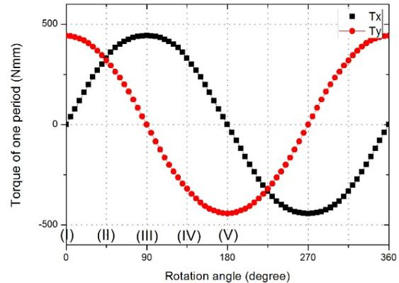
Figure 4: The torque per unit period for a PM cylinder undulator with dimensions as given in Table 1. The configurations (I) to (V) correspond to the orientations of the PM cylinders in Fig. 3.
