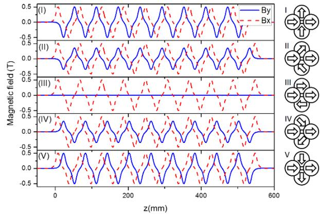
Figure 3: Change of the vertical ( $B_y$ ) and horizontal ( $B_x$ ) magnetic fields during helicity switching. Configurations (I) to (V) represent the orientations of the PM cylinders.
