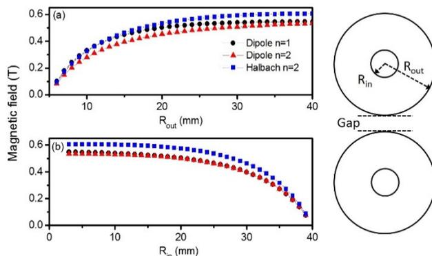
Figure 6: Simulating magnetic fields for the PM cylinder undulator versus dimensions of (a) outside radius and fixed  $R_{in} = 5\text{mm}$  and (b) versus inside radius at a fixed  $R_{out} = 40\text{mm}$ . Other parameters are from Table 1.
