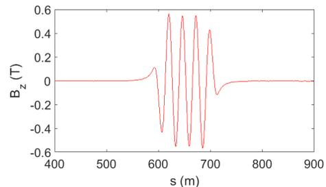
Figure 5: RTU B-field measurement result before installation.
