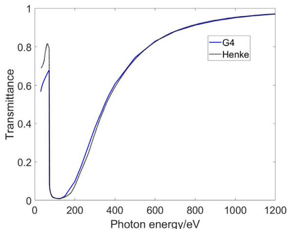
Figure 2: 150nm Aluminum foil transmittance
