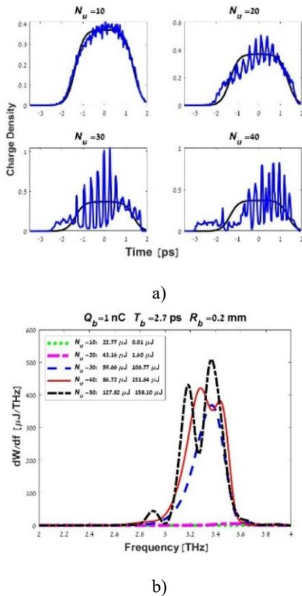
Figure 3: Evolution of bunch density (a) and high-frequency parts of radiation spectra (b) for an extended bunch with charge of 1 nC, radius of 0.3 mm, duration of 2.7 ps, and energy of 6 MeV passing the distance of (10-40) cm in un-dulator with period of 10 mm and waveguide with diameter of 1.5 mm.
