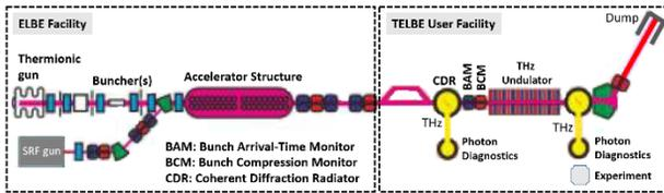
Figure 1: ELBE accelerator beamlines for THz radiation production.
