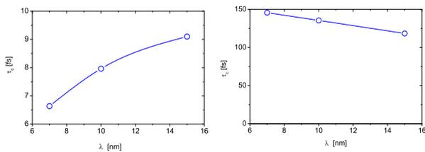
Figure 5: Coherence time (left) and radiation pulse duration (right) derived from the gain curves shown in Fig. 4.
