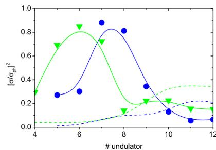
Figure 6: Ratio of dispersions of the full radiation pulse energy to that filtered by a pinhole,  $\sigma^2/\sigma_{ph}^2$  (solid lines). Dashed curves show relative fraction of the radiation power passed through a pinhole. Blue and green colors correspond to the radiation wavelength 10 nm and 15 nm.
