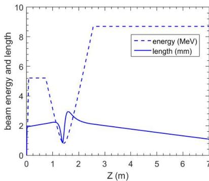
Figure 2: The evolution of the kinetic energy (dash line) and the rms beam length (solid line).
