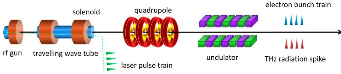
Figure 1: A schematic layout of the pre-bunched THz FEL based on velocity bunching.
