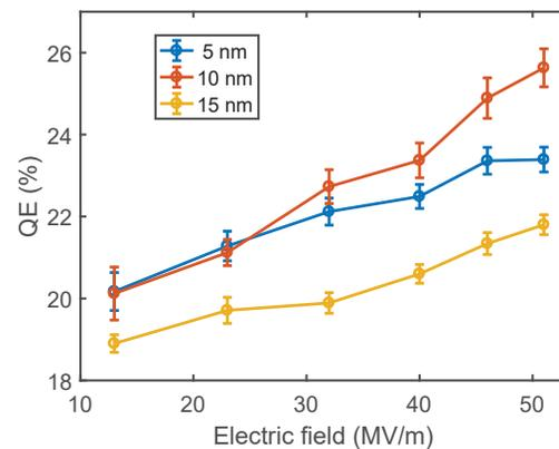
Figure 3: The plot of QE at the center of the cathode against electric field during emission for three cathodes. The error bars are the statistical error.
