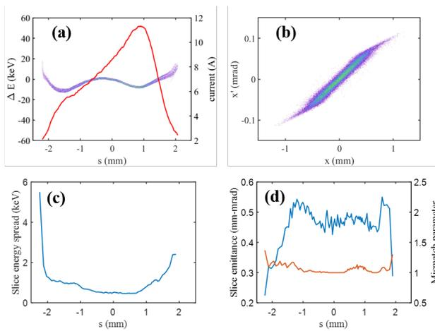
Figure 3: Electron beam distribution at the exit of the injector beamline. (a) Longitudinal phase space and current profile. (b) Transverse phase space. (c) Slice energy spread. (d) Slice emittance and mismatch parameter.
