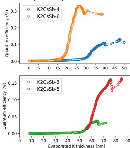
Figure 3: Comparison of QE @ 543 nm during K deposition. Upper plot “5 nm Sb”, lower plot “10 nm Sb”.
