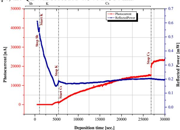
Figure 1: Photocurrent (red) and reflected power (blue) during deposition of cathode KCsSb-5. The incident power @ 543 nm during photocathode growth was 1.9 mW.
