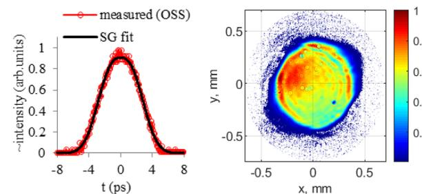
Figure 4: Left: Photocathode laser pulse temporal profile measured with OSS supplied with a Super Gaussian (SG) fit  $SG \propto \exp\{-0.5 \cdot |t/2.6|^{2.59}\}$ . Right: Transverse distribution of the laser intensity for the BSA diameter of 0.8 mm: laser RMS sizes:  $\sigma_{x/y}^{laser} = 0.196/0.200$  mm.
