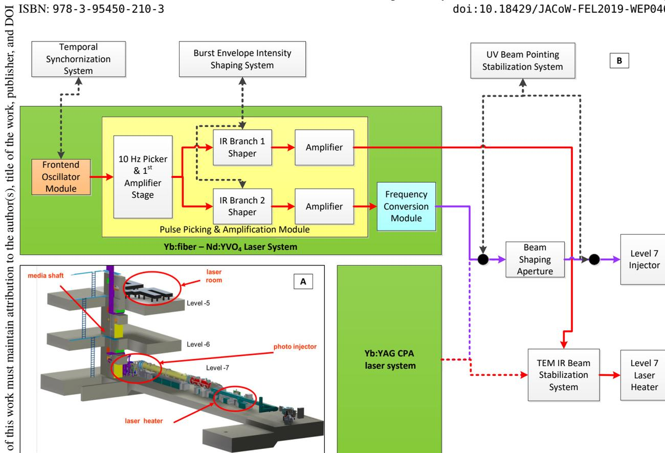
Figure 1A: Injector Building Layout, 1B: Injector Laser System.
