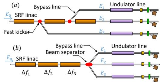
Figure 1: Two schemes of multi-energy operation of a SRF XFEL: (a) kick the beam to bypass line at desired energy point (b) control the beam energy independently by off-frequency detune of SRF cavities.
