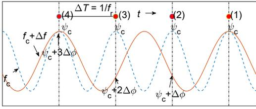
Figure 2: Acceleration phase changes of the CW electron beams by the off-frequency detune of the SRF cavities. Here we use  $M = 3$  and acceleration phase of the fourth beam is the same with the first one.
