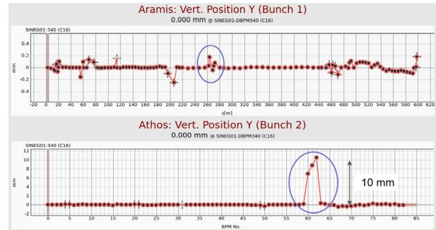
Figure 4: Vertical position of the two bunches during bunch-separation: upper graph – “Bunch 1” through Aramis beamline and lower graph – “Bunch 2” through Athos.
