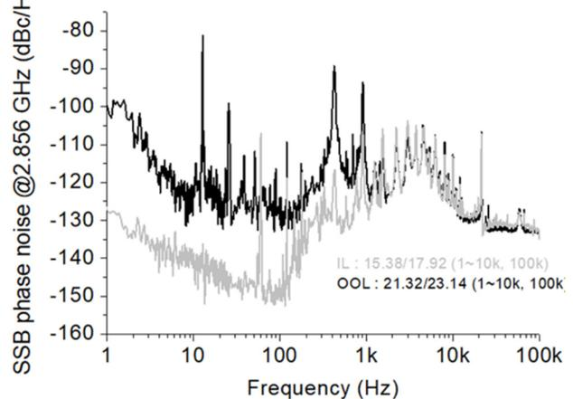
Figure 5: Measured relative phase noise between RF and optical pulse train after synchronization. IL : in-loop, OOL : out-of-loop.
