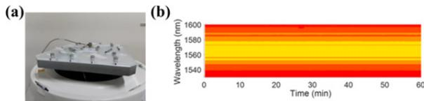
Figure 2: Vibration test of all-PM-fiberized 3 x 3 coupler based NALM laser. (a) The shaker generates 1.5g<sub>rms</sub> vibration and (b) optical spectrum from the port 1 is recorded for >1 hour. Note that the data and figure are based on [3].
