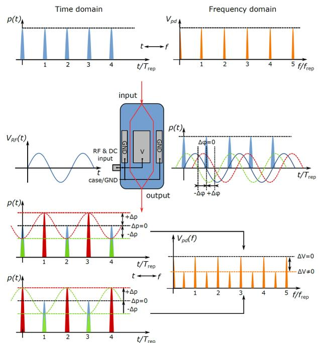
Figure 5: Concept for Mach-Zehnder modulator based laser-to-RF synchronization scheme. Blue pulses indicate the unmodulated optical pulses in time domain, red and green pulses depict the modulated optical pulses in time domain. Orange comb lines show the frequency spectra for both modulated and unmodulated optical pulses.
