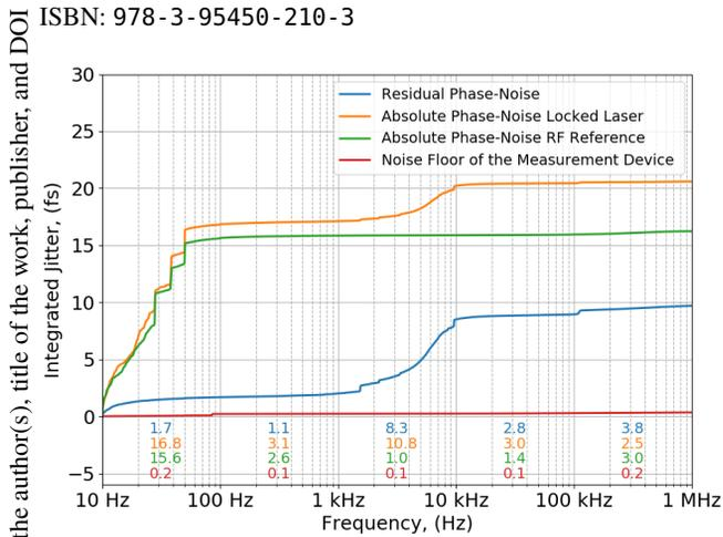
Figure 4: Integrated timing jitter calculated from the phase-noise PSD in Fig 3.
