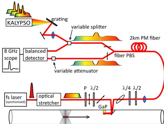
Figure 2: Schematic drawing of a spectrally encoded electro-optical detection setup including the single shot spectrometer and the photonic time-stretch detector. P: polarizer; PBS: polarizing beam splitter.
