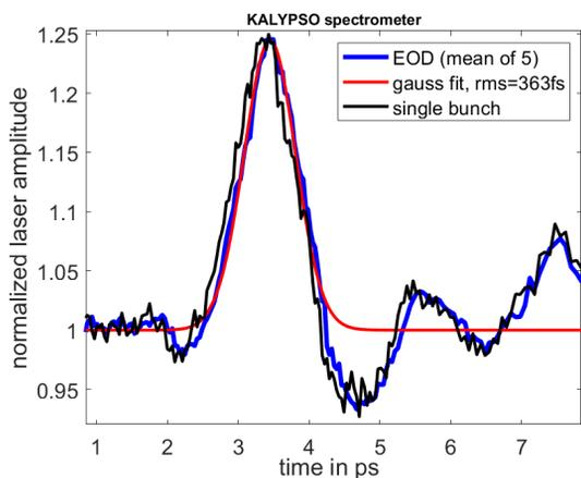
Figure 4: A single-shot EOSD measurement from the spectrometer with the EOD setup before modification showing a significantly better SNR. Here the bunch charge was 500 pC.
