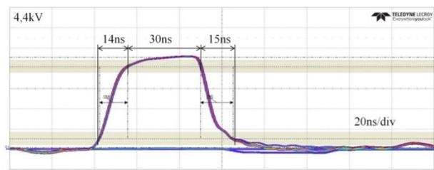
Figure 3: Scope screen showing overlaid pattern of pulses with stable flat top and non-ripple baseline.
