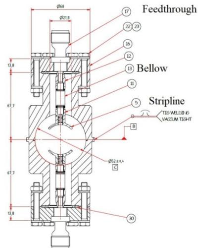
Figure 2: European XFEL KS dump kicker cross section.
